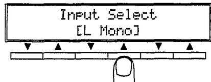
NOTE: When you select the input mode to be "L Mono" signal or "R Mono" signal even when connecting both the L and R terminals, monaural input signals will be transmitted.
