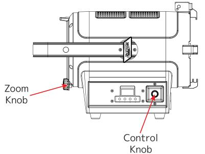
**ZOOM KNOB:** Manually adjust the zoom of the fixture in and out.
